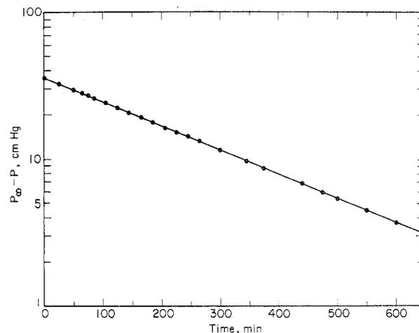
**Figure 3.** Semilogarithmic plot of  $P_{\infty} - P$  vs. time for the hydrolysis of  $\text{B}_3\text{H}_7\text{OH}_2$  in 88% methanol-12% water at  $-45^\circ\text{C}$ , with 1.25 M HCl.
