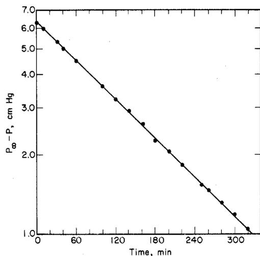
**Figure 1.** Semilogarithmic plot of  $P_{\infty} - P$  vs. time for the hydrolysis of  $\text{KB}_3\text{H}_8$  in 88% methanol-12% water at  $-78^\circ\text{C}$ , with 1.25 M HCl.
