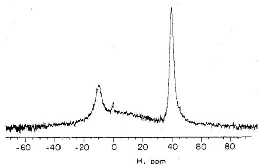
Figure 4. Boron-11 NMR spectrum of  $B_3H_7OH^-$  in 88% methanol-12% water at  $-65^\circ C$ .
