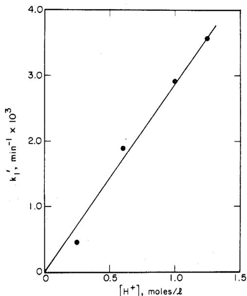
**Figure 2.** Plot of pseudo-first-order rate constant  $k_1'$  vs. hydrogen ion concentration, for hydrolysis of  $\text{KB}_3\text{H}_8$  in 88% methanol-12% water at  $-78^\circ\text{C}$ .
