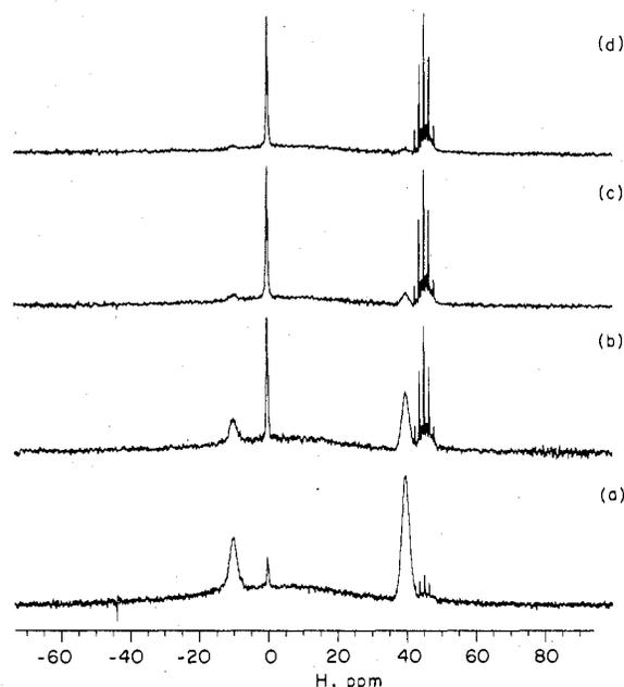
Figure 5. Boron-11 NMR spectra of decomposing  $B_3H_7OH^-$  solution: (a) after 2 min; (b) after 30 min; (c) after 2 h; (d) after 3 h.
